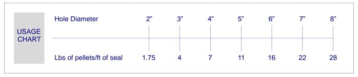
NOTE: These are dry weights and volumes. In use, the swelling of the pellets will increase the length of the seal (depending on hole condition).
